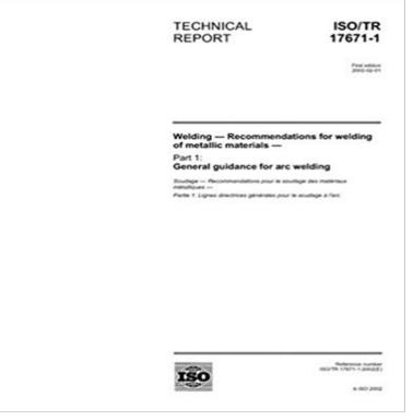
ISO/TR 17671-1 gives general guidance for fusion welding of metallic materials in all forms of product (e.g. cast, wrought, extruded, forged). The processes and techniques referred to in this part of ISO/TR 17671 may not all be applicable to all materials.
